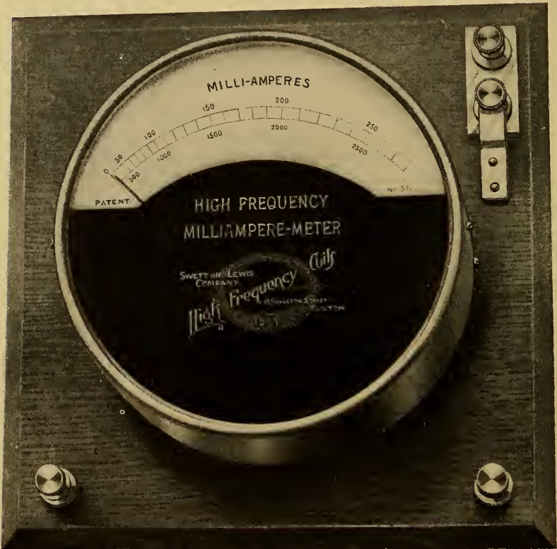
FIG. 104.—Hot Wire Milliamper Meter for Measuring the Intensity or Volume of Currents of High-frequency.
